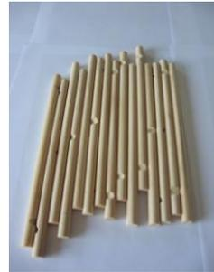
2: Take 10 of the dowels. Then using a round rasp or round file, create three notches into each of the 10 dowels.
